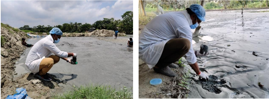
Figure 18: River Bed and Dredge Material Sampling at Lot3 and Lot2 Sites Respectively
