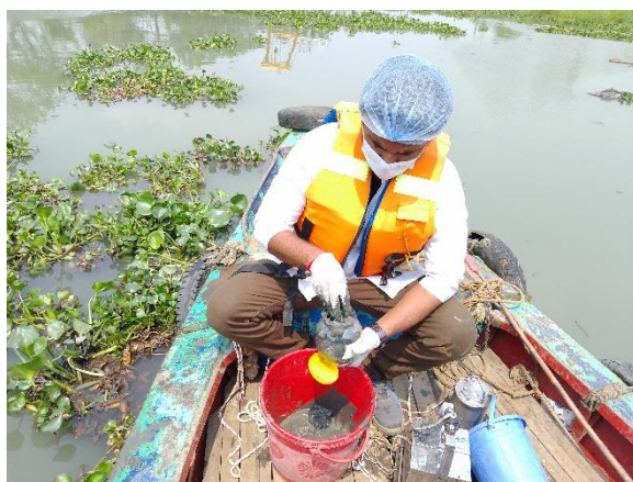
Figure 5: Riverbed sediment sampling at Solimganj ghat
